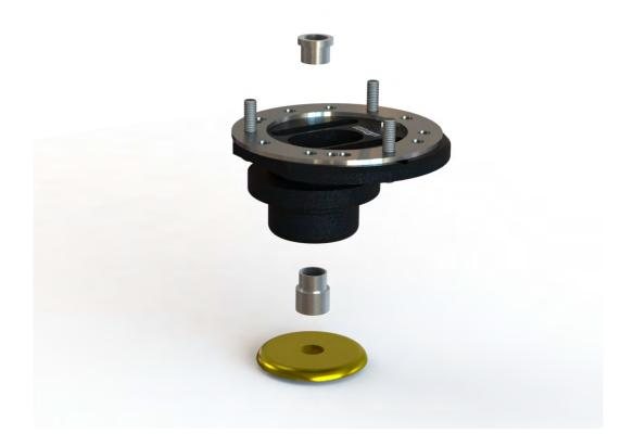
Remove the original spring plate and mount it on the bearing housing. Use the large OEM washer and the spacers as illustrated.
